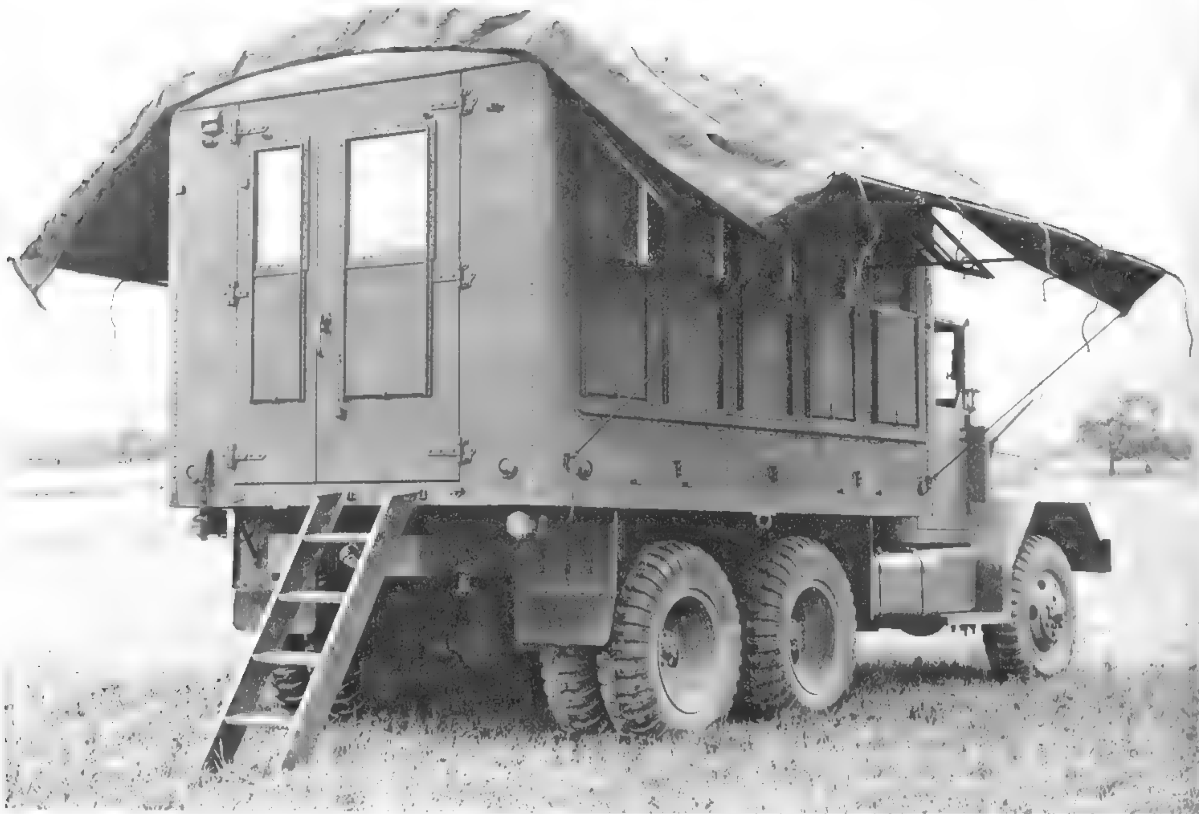
The M109 canvas could be used as an awning, reducing the temperatures inside the van. (National Archives and Records Administration photo)
